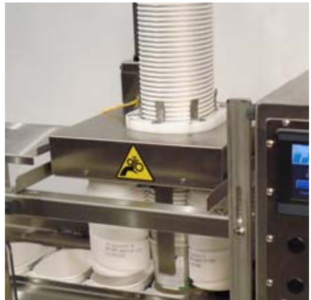
Servo Driven Progressive Pitch Auger Denester
