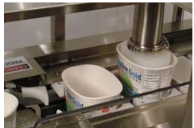
Servo Driven Split Pocket Container Indexer
